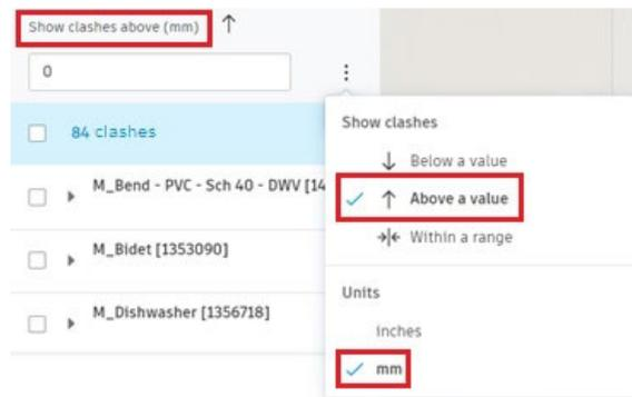
When you mark one of the clashes shown in the list, the 3D view is automatically positioned to show the element that is in potential clash.
