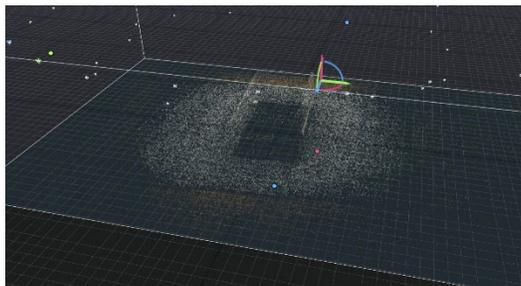
After obtaining the point cloud, we continue with the *mesh* processing, therefore, we access to the section **MESH MODEL** and select the *normal detail* option, if the alignment has been satisfactory, the reconstruction of the polygonal mesh does not require the settings to be retouched.
