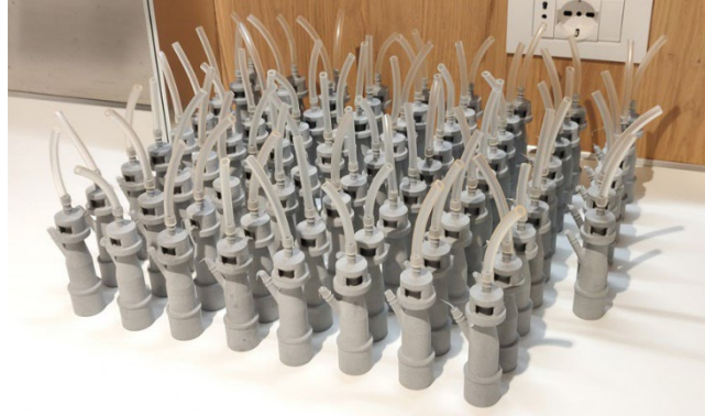
3D printed valves. Source: 3DNatives.
