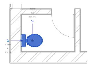
When clicking on the inserted equipment, the Properties Palette identifies the object and customized changes can be made according to each project. Next to the object, the identifications of the water inlet and outlet connectors appear.
