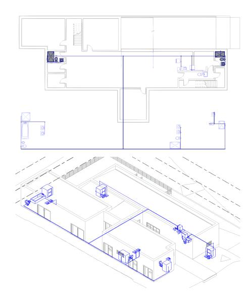
With the Domestic Cold Water system already structured in the project, a pipe must be drawn to connect the system with the point of the public network. In this project, the location of the public network point is not represented, therefore, an approximation will be made.
