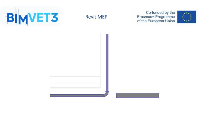
Delete the existing connection between the two pipes, click the end of the pipe horizontally and drag it to meet the new 40mm pipe.
