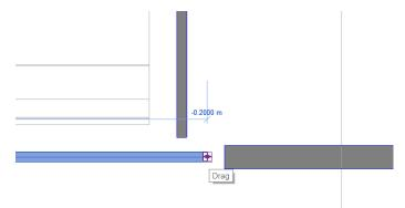
A connection will be automatically created between the two pipes, with the diameter reducer (from 40 mm to 15 mm) coupled.
