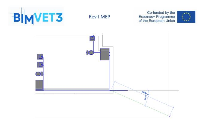
After extending the pipe, click on it to select it. On the Modify | Pipes, Edit panel, select the Cap Open Ends option, to close the unconnected end of this pipe, as the connection to the public network is made by the local water company.
