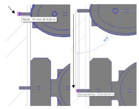
The pipe that goes under the toilet will also be deleted and a new one will be drawn with the Pipe tool so that it lines up with the pipe at the other end.
