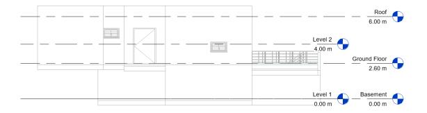
It is recommended that Level 1 and Level 2 are renamed "Basement" and "Ground Floor", respectively, and that their heights be changed so that they are on top of the levels of the imported design (0.00 m and 2.60 m). A third level should be created and named "Roof", with a height of 6.00 m.
