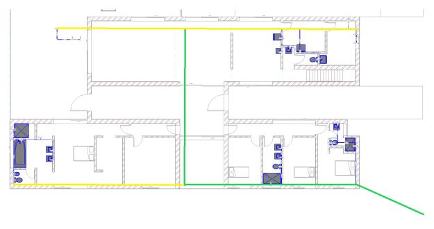
The change is made in a very simple way. Just click on the pipe to be changed and in the Options Bar (Modify Pipe) in the Diameter parameter, select the desired value (25mm or 40mm).
