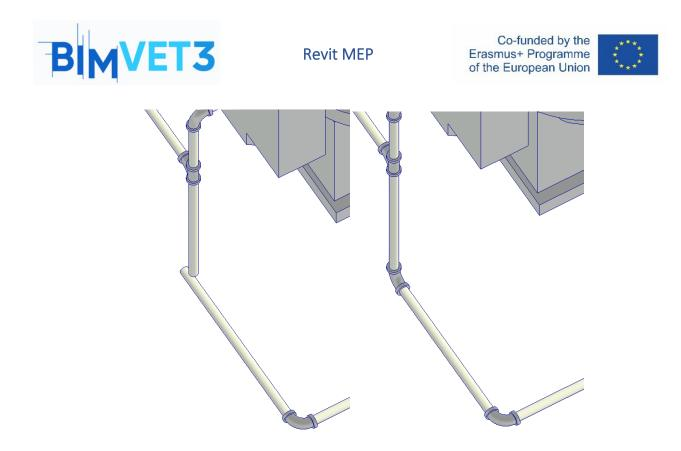
The other equipment will also be connected in a more optimized way, such as the washbasins. This type of washbasin has a diameter of 25 mm for the inlet of cold water. You must change this measurement by clicking on the element and in the Properties Palette click on Edit Type.
