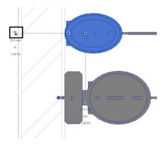
Then, a line that represents the piping path appears, which moves according to the movement of the mouse cursor. Observe the temporary dimension and insert 0.10 m into the wall.
