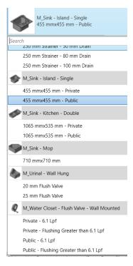
For this example, none of the devices that initially appear in the Type Selector list will be used, as new families will be loaded. To do this, after clicking on the Systems tab and the Plumbing Fixture icon, the Modify |Place Plumbing Fixture tab will open, and so click on Load Family.
